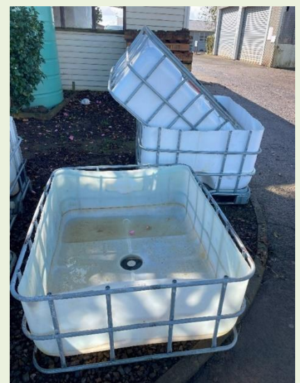
The base of the IBC includes a built-in pallet for easy movement by forklift. The top half, however, requires the addition of a pallet to facilitate similar mobility.
